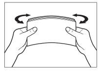
② Place the envelopes on a clean, level surface, and press all the way around the envelopes by hand, in the direction of the arrows, to remove any curls. Repeat this step five times for each set of five envelopes.
